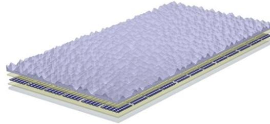
*Pyramid:* 45° base angle and height of 1 mm
