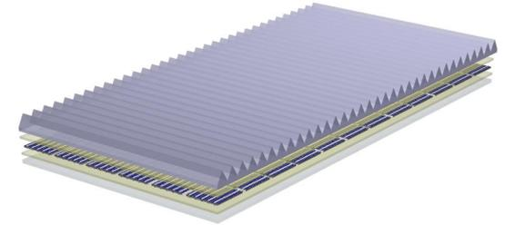
*V-Grooved:* V-grooves parallel to short edge with a 50° base angle
